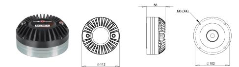
220 W continuous program power capacity 1.4" horn throat diameter 75 mm (3 in) aluminum voice coil Titanium diaphragm 500 - 18000 Hz response 109 dB sensitivity Neodymium magnet assembly with shorting copper cap
