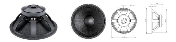
2400 W continuous program power capacity 100 mm (4 in) copper voice coil 35 - 1000 Hz response 94 dB sensitivity Aluminium demodulating ring allows a very low distortion figure Double silicone spider with optimized compliance
